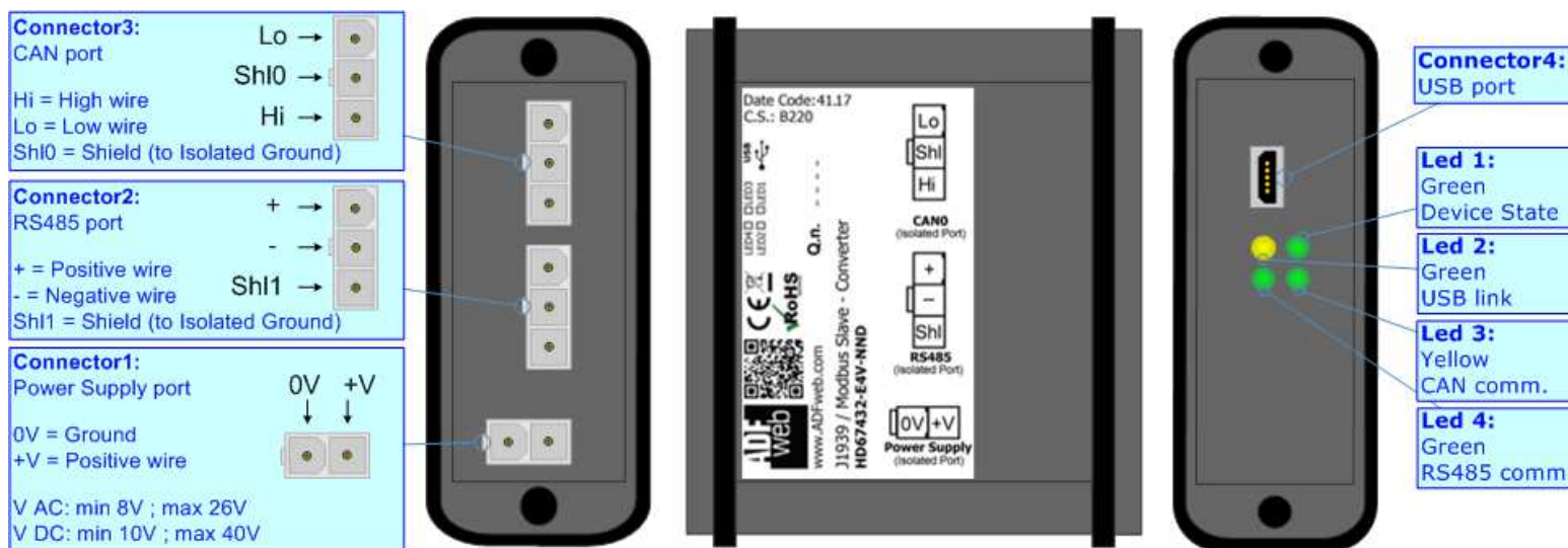
Figure 1a: Connection scheme for HD67432-E4x-xxx
