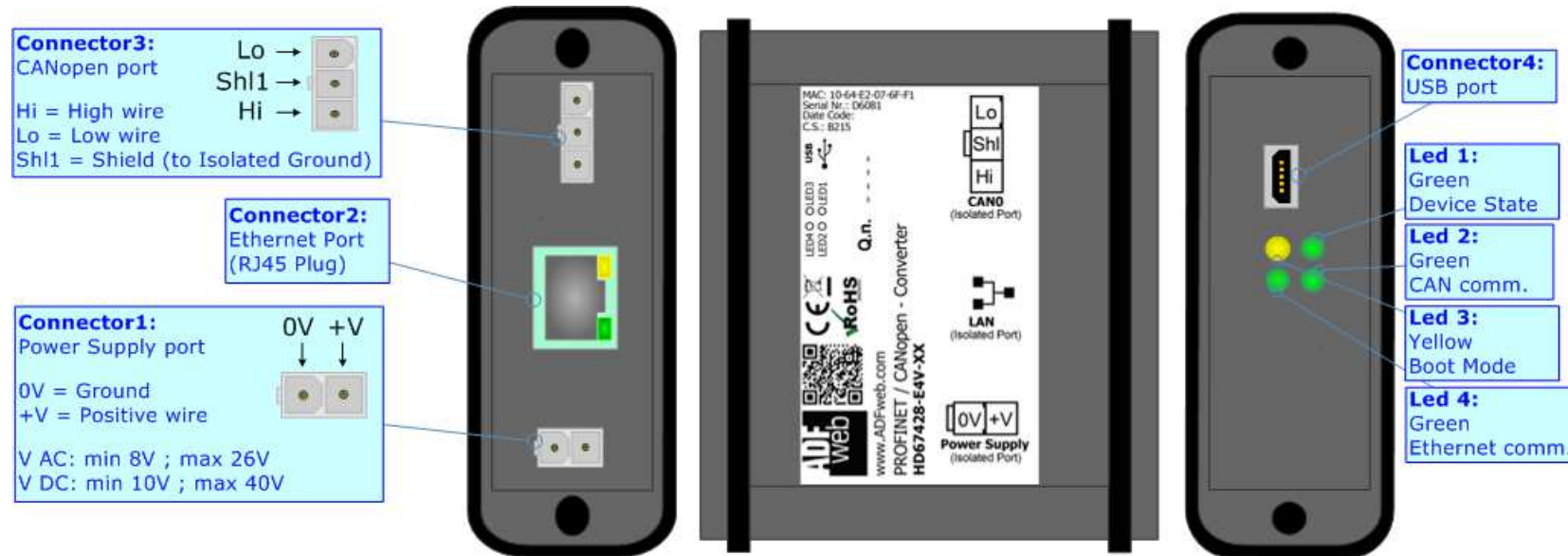
Figure 1a: Connection scheme for HD67428-E4x-xx
