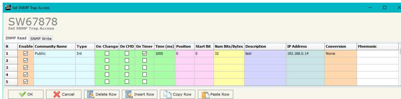
Figure 13a: “Set SNMP Access -> SNMP Read” window
