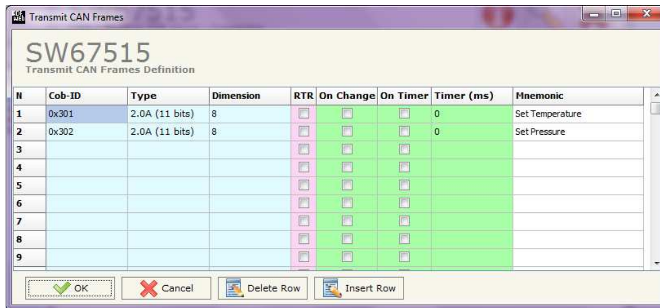
Figure 6b: "Transmit CAN Frame Definition" window
