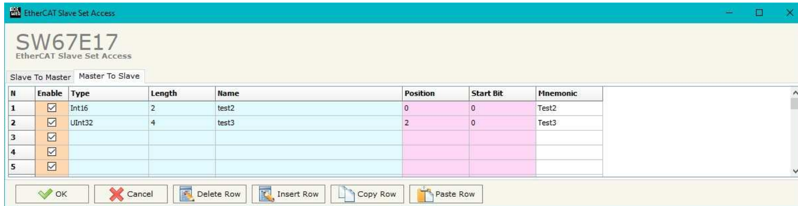
Figure 4b: "EtherCAT Slave Set Access → Master To Slave" window
