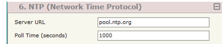
Figure 3h: “Set Communication → NTP” window
